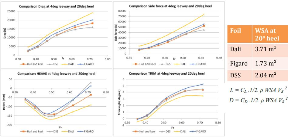
Example of graph for upwind condition at high heel angle
