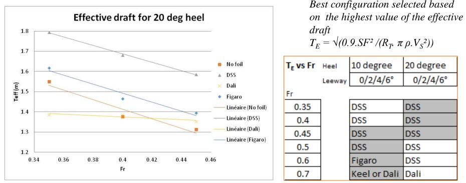
Example of graph for upwind condition for high heel angle
