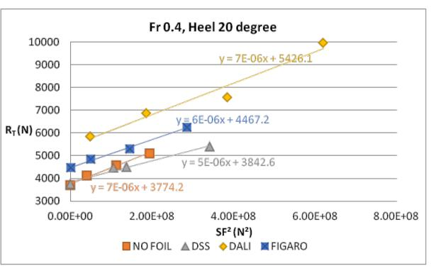
Best configuration selected based on the lowest slope:  $y/x = R_T / SF^2$
